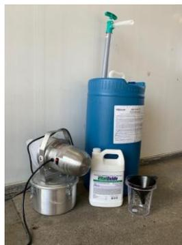
1. Remove Fogger power head from tank and add 5-7 oz. Vital Oxide solution to fogger tanks and fasten clamps to secure power head
